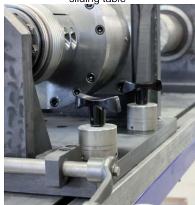
MCA-T power clamping nut for adjustment of test bench sliding table
