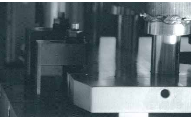
Slide-in Clamp device MES for clamping the upper and lower die in a Spotting Press
