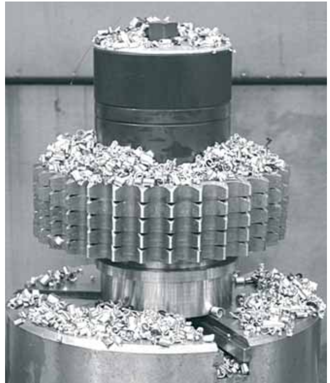
Clamping nut MCA for clamping of chain wheels during milling
