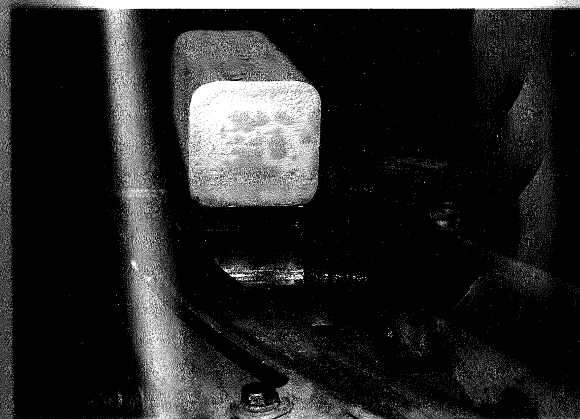
100 BILLET ENDS - SAWED VS. BROKEN 101 SAWED BILLET AFTER ATMOSPHERICALLY-CONTROLLED HEAT TREAT - NOTE MINIMUM SCALE
