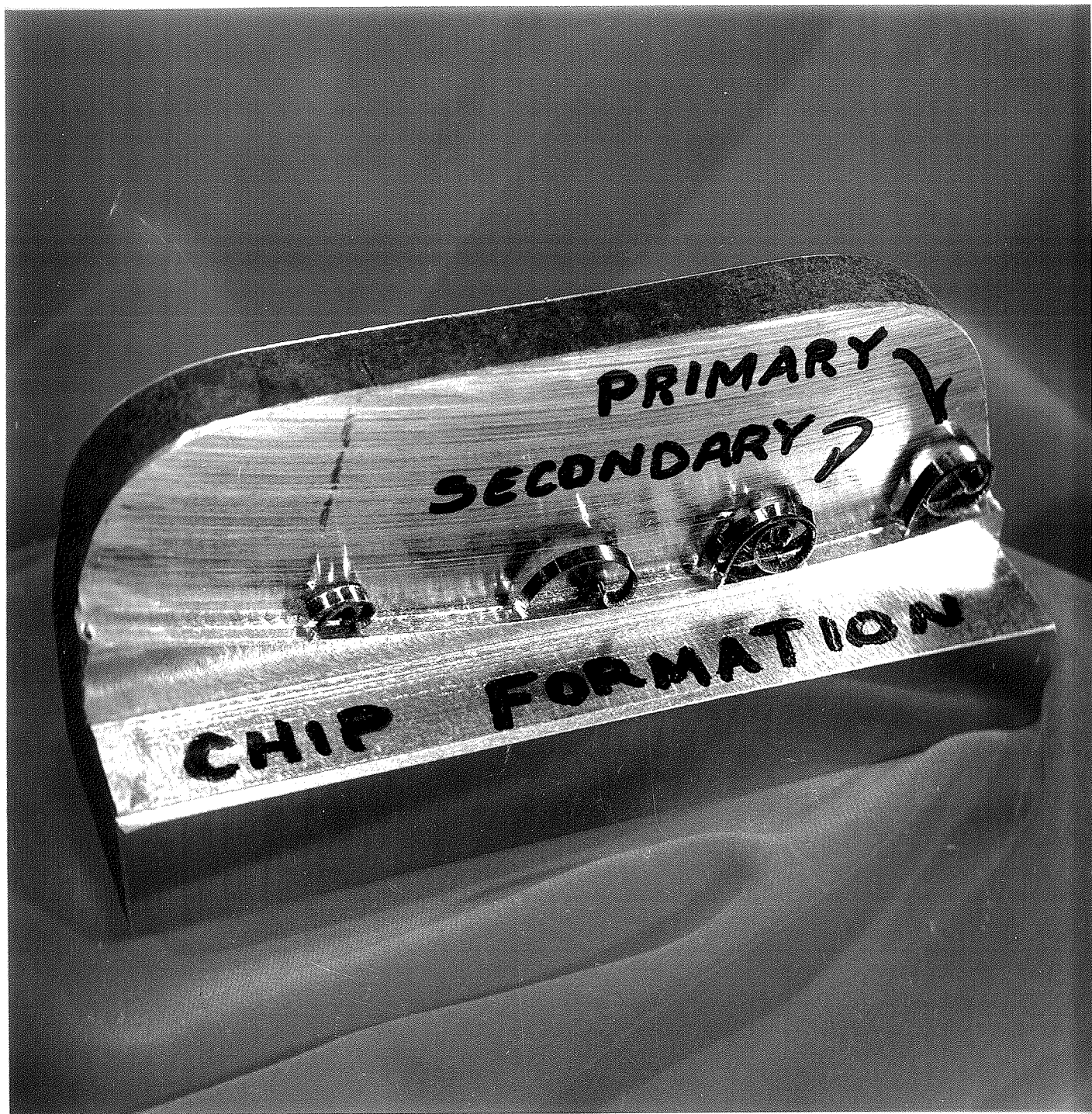
Photo No. 1453 CUTAWAY VIEW OF WAFER ILLUSTRATING CHIP FORMATION
