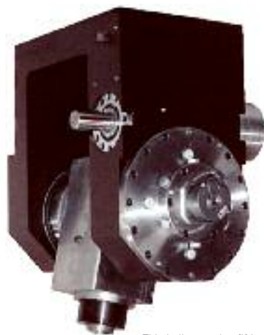
This built-to-order, fifth-axis milling head was created for a traveling gantry and features a motorized precision spindle operated by a zero-backlash OTT Worm Drive with encoder and programmable controller.
