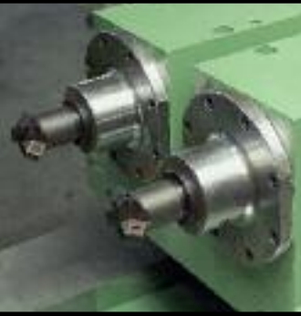
Amsaw rail drill chamfers.
