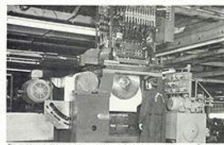
Structural steel will be cut using a carbide saw for the first time in Japan using two Metalcut saws like the one above. The fast growing Rockford, Ill. firm is also planning to introduce a new 18-in. carbide saw during the next national machine tool show.
