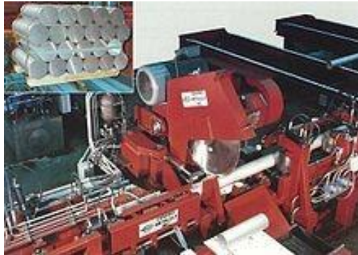
Fully automatic saw system with a Metalcut XII-P Aluminum Pivot Saw
