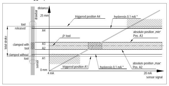
\* The limits are exactly adjusted. A hysteresis of 0,1 mA (equals approx. 0,15 mm) accounts for existing tolerances e.g. thermal expansions. However, this hysteresis is programmed only for the positions "tool released" and "clamped without tool". No additional tolerance has to be considered!
