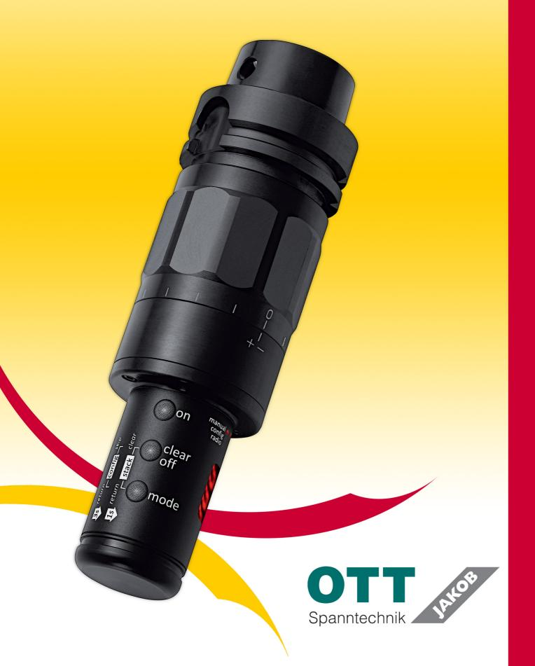
The **POWER-CHECK II** is a measuring device used to check the force with which the tool pulled into the spindle taper. The specified pull force is very important for the quality of machining. Including the **POWER-CHECK II** into your preventive maintenance schedule will allow you to notice a reduction of the pull force and prevent the above mentioned problems before they occur.
