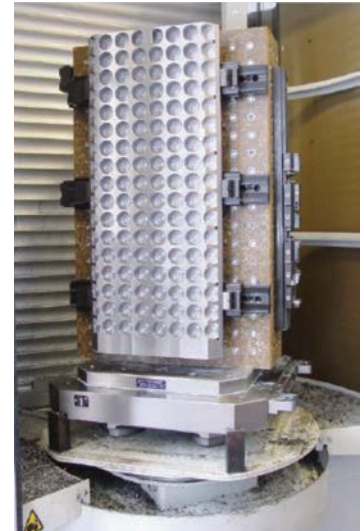
Large part clamping.
