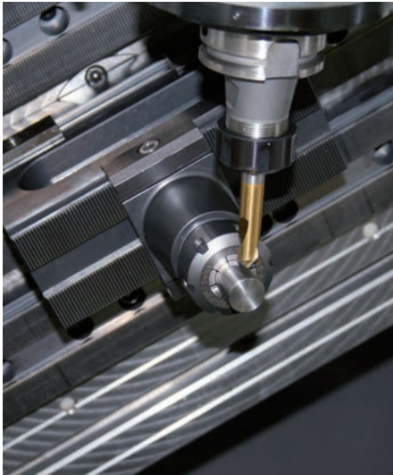
Collet chuck ER32 in operation.
